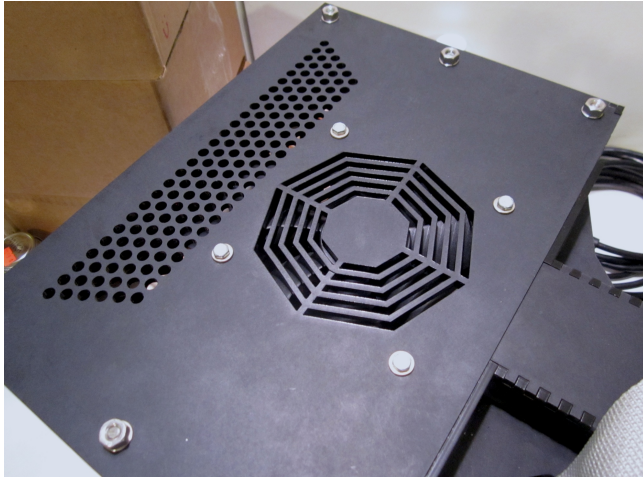
Figure 4: A cooling fan installed on the top of the projector pod.
